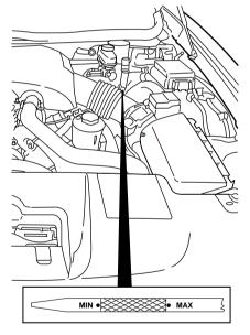
6. Wipe the indicator clean. Insert the indicator fully, then remove it again.
